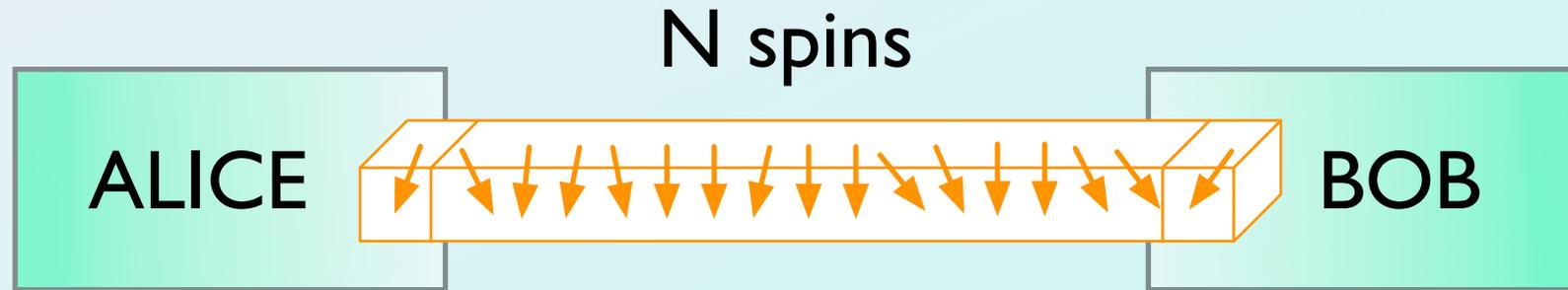
*Linear chain of permanently coupled spins*
